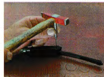
3-Remove the firing pin retaining pin from the bolt assembly, while holding the firing pin and firing pin spring in place
