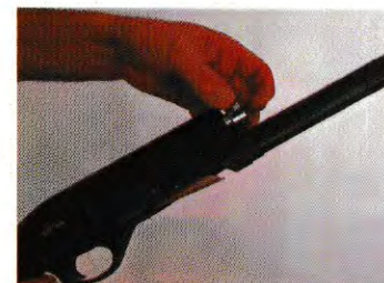
2-Take out the charging handle and the bolt group.
