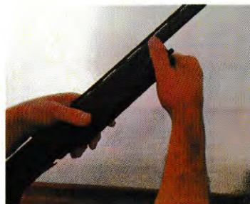
1-Unscrew the magazine cap and take out the forend and barrel group by sliding forward.
