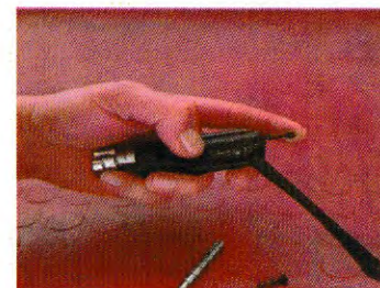
3-Remove the firing pin retaining pin from the bolt assembly, while holding the firing pin and firing pin spring in place
