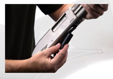
Push the forearm forward and close the action. Push a shell upward againts the bottom of the carrier and then forward to install a shell in the magazine tube. Repeat this step until the tube is full or you've achieved the desired number of shells.
