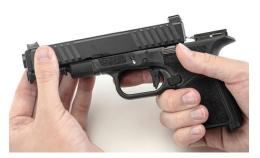
STEP 4: SIMULTANEOUSLY, PULL DOWN AND HOLD BOTH SIDES OF THE SLIDE LOCK USING THE THUMB AND INDEX FINGER OF YOUR FREE HAND. PUSH THE SLIDE FORWARD UNTIL IT IS FULLY SEPARATED FROM THE RECEIVER. PUSH THE RECOIL SPRING ASSEMBLY SLIGHTLY FORWARD WHILE LIFTING IT AWAY FROM THE BARREL.
