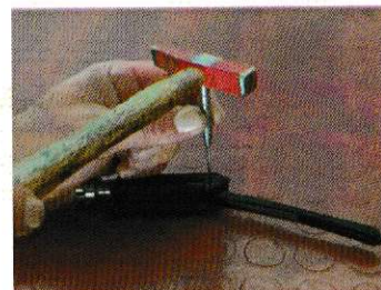
3-Remove the firing pin retaining pin from the bolt assembly, while holding the firing pin and firing pin spring in place
