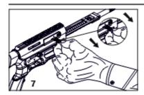
Pull back slightly on the bolt carrier to center the charging handle down in its slot for removal.
