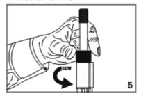
Remove the operating rod nut in the direction of the arrow.
