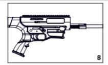
8) Push the bolt and carrier to the rear and engage the bolt stop to hold the bolt in the "open" position. Be careful to not allow the bolt to fly forward.
